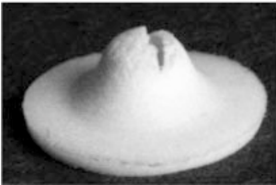
Figure 11.18 Micrograph of a deformed and failed specimen used in a small punch test.
