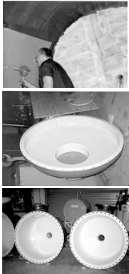
Figure 8.2 Adhesively bonded lining: (top) thermoforming of sheets, and (middle and bottom) finished lined head. (Courtesy Electrochemical Engineering and Manufacturing Company.)
