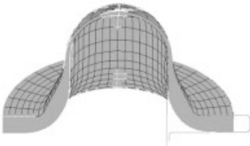
Figure 11.19 Example of deformed mesh used to simulate a small punch experiment.
