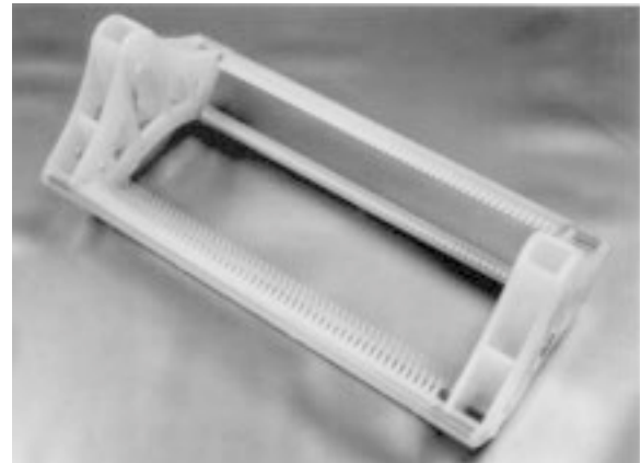
Figure 6.38 A semicon wafer carrier-fusion bonded assembly of injection molded side rails and strengthened by pultruded rods consisting of carbon fiber compounded PFA. (Courtesy Entegris and DuPont Companies.)
