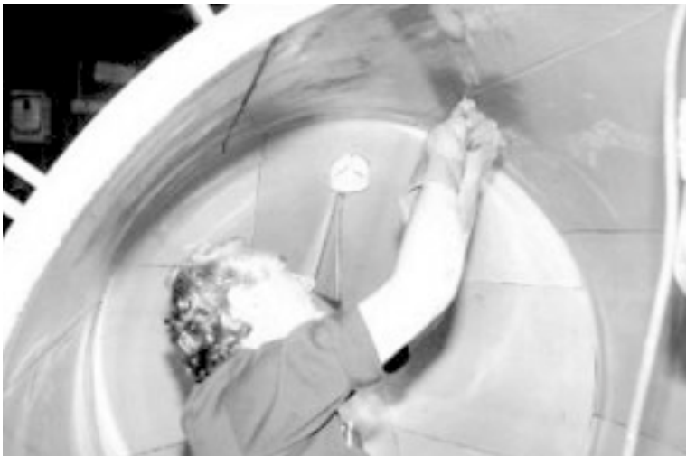
Figure 8.3 Preparation of the lining for root pass. (Courtesy Electrochemical Engineering and Manufacturing Company.)
