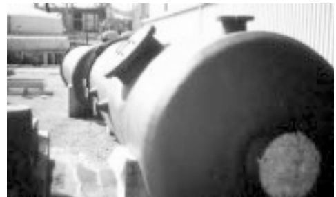
Figure 8.27 Dual laminate scrubber column with ETFE Tefzel®. (Courtesy RL Industries and DuPont Company.)
