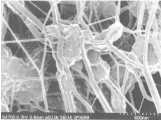
Figure 5.26 An example of biaxially oriented fibrillated PTFE structure. (Courtesy of Mr. Clay Jones, DuPont Fluoroproducts.)
