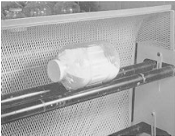
Figure 5.28 Blending fine powder PTFE by bottle rolling. (Courtesy DuPont.)
