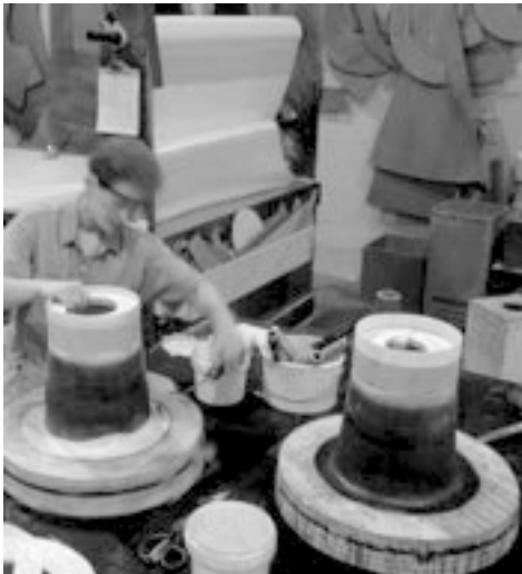
Figure 8.25 Dual laminate flange fabrication. (Courtesy CPF Dualam.)
